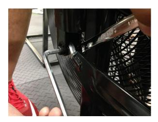
5. **Chain Adjusting Check (Quarterly)**: Check the two drive chains to make sure they are equally tight. Each chain should have just a slight flex to it, but it should also not be tightened too much. First check the main rear chain and adjust the tension if needed. Proper chain tension is about 3mm of movement up and down or a slight up and down movement.
